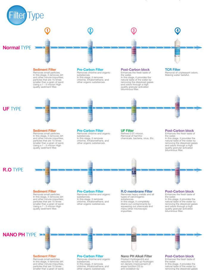
smaller than a grain of sand. Using a 1 - 5 micron High quality sediment filter.
